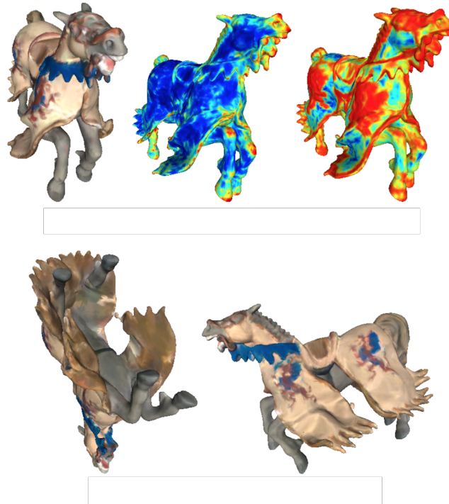
FIGURE 3 – Optimal viewpoint selection for colored meshes. First line, from left to right : original colored mesh, geometry-based saliency, the proposed global geometry and color saliency. Second line : Optimal viewpoint based on geometric saliency, optimal viewpoint based on global saliency.
